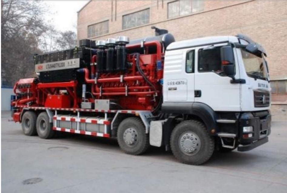
The Lanzhou Shengda 3000 fracturing truck is equipped with an Allison 9832 Oil Field Series™ transmission. Its lightweight and compact size is ideal for the truck's compact dimensions. (Photo: Business Wire)
