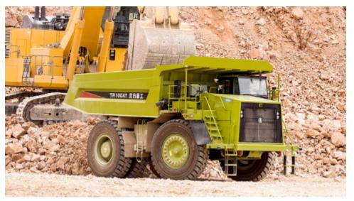
Inner Mongolia North Hauler Joint Stock Co., Ltd (NHL) NTR100A autonomous driving dump truck equipped with an Allison 8610ORS automatic transmission. (Photo: Business Wire)
