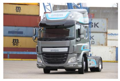
The EMOSS Electric Vehicle with Extender Range (E.V.E.R.) semi-truck utilizes a 120 kilowatt-hour (kWh) battery pack and a liquefied petroleum gas electricity generator to recharge the battery and achieve maximum range. It is further equipped with an Allison 4500 fully automatic transmission and rated for a gross combination weight of up to 50 metric tons.
