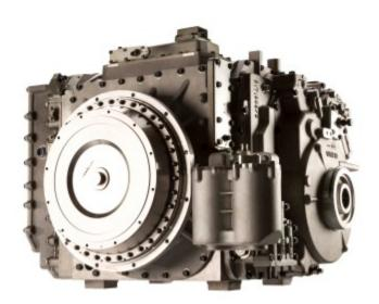
Allison engineers also have a track record of retrofitting existing models. A recent example is the ongoing testing of a Bradley Fighting Vehicle now outfitted with the 3040 MX (pictured), a variant of the X300<sup>™</sup>, found in the British Warrior, British Terrier and Swedish CV90 vehicles. (Photo: Business Wire)
