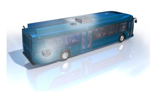
The Allison eGen Flex<sup>™</sup> can operate in full engine-off mode up to 50% of the daily duty cycle of a transit bus. It is capable of operating in electric-only mode for up to 10 miles or 50 minutes, multiple times per route and per day. (Photo: Business Wire)
